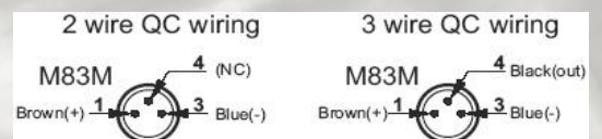
M8 Quick Connector (IEC61076-2-101)
